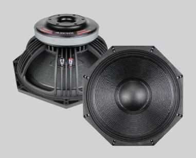
Thiele & Small Parameters: Fs: 36 Hz Re:  $4.5 \Omega$  Qes: 0.30 Qms: 6.83 Qts: 0.29 Vas: 201.66 L Cms: 0.09 mm Sd: 0.12 m2 Mms: 199.2 g Xmax: 15 mm Bl: 25.9 T.m Le(1KHz): 1.43 mH
